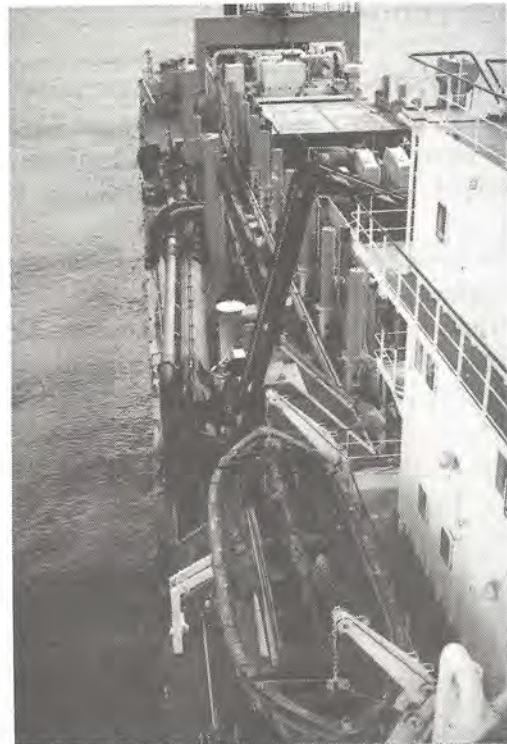
Fig 3.26: The dredge arms of the trailing suction dredge, Ham 310 off Kirra 1990
