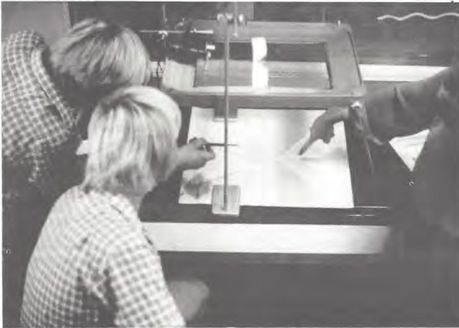
Fig 1.40: A ripple tank set up
