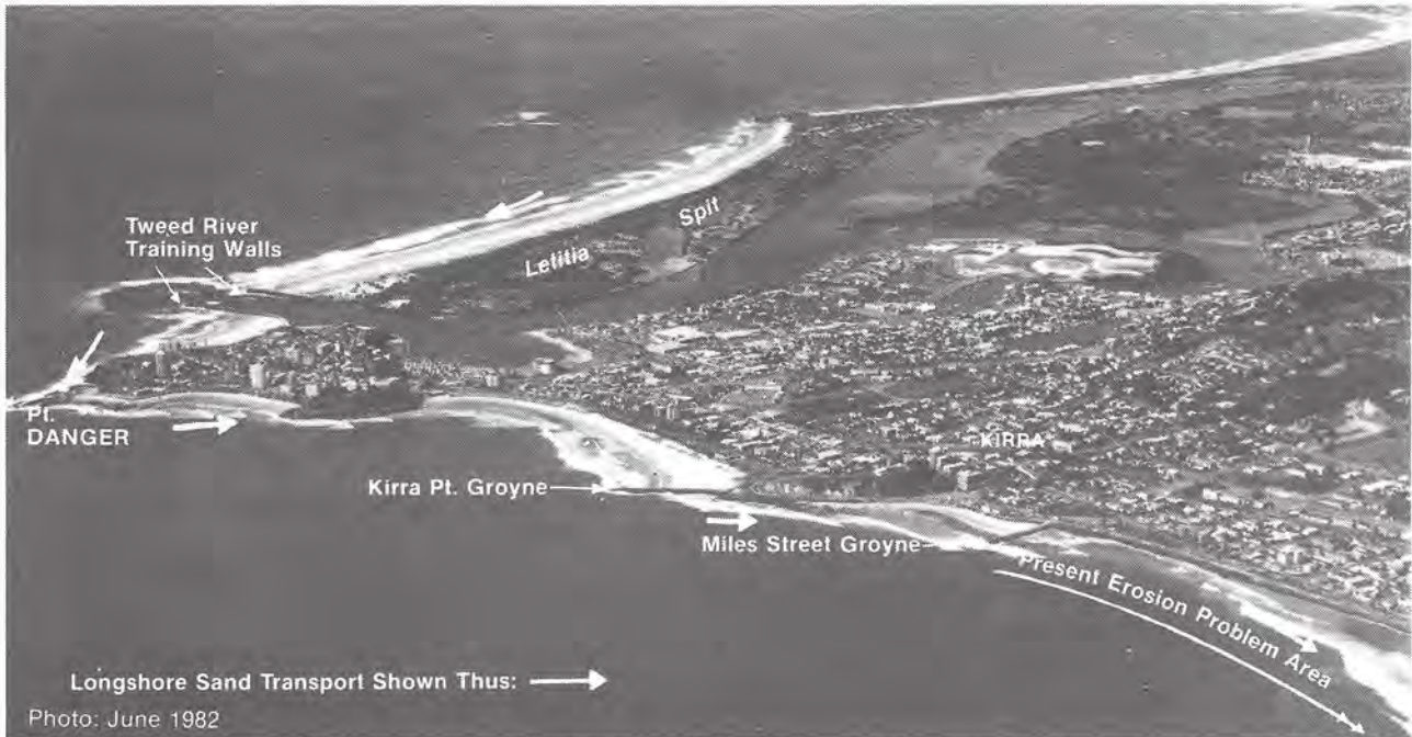
Fig 3.21: Groynes were used to stabilise the beaches as a temporary measure. Long term solutions to this problem were to cost millions of dollars. Photograph courtesy Beach Protection Authority.
